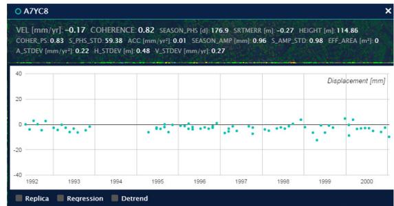
Data is available from 1992 to 2000 and includes velocity, season, area, height, coherence and a range of standard deviations. Ground displacements are shown as a row of dots with movement in mm.
