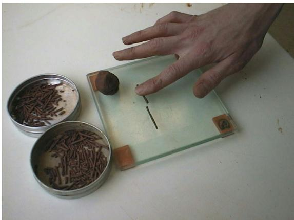
*Rolling out threads of soil to determine whether they crumble beyond a particular moisture content is at best crude and of limited reliability. Any notion of 'accuracy' is mute given the changes in structure and mineralogy over just a few metres in the ground. We simply need to know if the soil undergoes volumetric change in relation to its moisture content and the LL test is more reliable and sufficient for our needs.*
