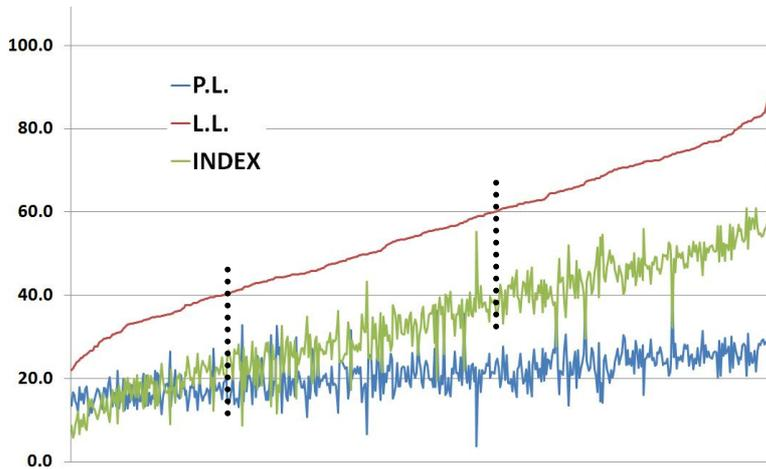
What is clear is that the Plastic Limit increases with the LL and although there is some scatter (see insets below main graph), the 'noise' doesn't change the fact that, in general, the LL is all that is needed to assess whether a soil is shrinkable and the broad category in terms of low, medium, high etc.
